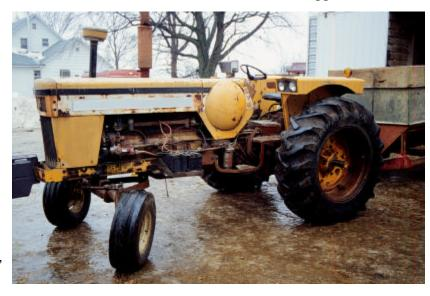
with the ignition key in the on position. The tractor originally had a safety switch built-in to the transmission, but it had been bypassed by the previous owner of the tractor. This enabled starting the tractor in gear when the clutch was pressed down.
